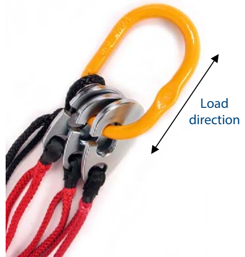
Lanyards with G-Hooks correctly attached to master link
